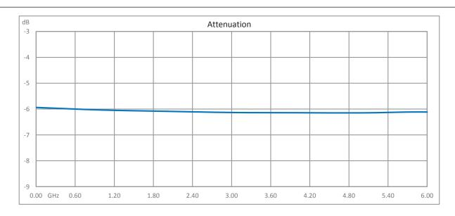
6 dB Fixed Attenuator SMA Male (Plug) To SMA Female (Jack) From 0.009 MHz To 6 GHz Rated To 2 Watts, Copper Body, 1.07 VSWR from Fairview Microwave is in-stock and available to ship same-day. All of our RF/microwave products are available off-the-shelf from our ISO 9001:2008 certified facilities in Lewisville, Texas. Fairview Microwave is RF on-demand.
