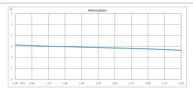
3 dB Fixed Attenuator SMA Male (Plug) To SMA Female (Jack) From 0.009 MHz To 6 GHz Rated To 2 Watts, Copper Body, 1.15 VSWR from Fairview Microwave is in-stock and available to ship same-day. All of our RF/microwave products are available off-the-shelf from our ISO 9001:2008 certified facilities in Lewisville, Texas. Fairview Microwave is RF on-demand.
