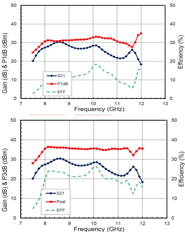
\*Bias at:  $V_{ds1,2,3}$  =+5V,  $V_{gg}$  = -2.6V,  $I_{dsq1}$ =0.14A,  $I_{dsq2}$ =0.56A,  $I_{dsq3}$ =1.3A.
