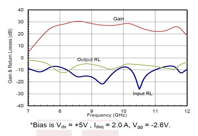
High Power GaAs Amplifier at 4 Watt Psat Operating from 8 GHz to 11 GHz with SMA from Fairview Microwave is in-stock and available to ship same-day. All of our RF/microwave products are available off-the-shelf from our ISO 9001:2008 certified facilities in Lewisville, Texas. Fairview Microwave is RF on-demand.
