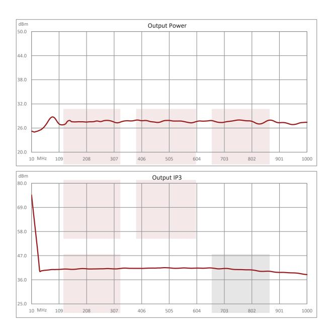
1.3 dB NF Low Noise Amplifier, Operating from 10 MHz to 1 GHz with 34 dB Gain, 27 dBm P1dB and SMA from Fairview Microwave is in-stock and available to ship same-day. All of our RF/microwave products are available off-the-shelf from our ISO 9001:2008 certified facilities in Lewisville, Texas. Fairview Microwave is RF on-demand.
