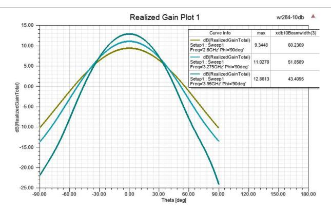
WR-284 Standard Gain Horn with 10 dBi gain, N Female Connector, with Pre-Installed L Mount from Fairview Microwave is in-stock and available to ship same-day. All of our RF/microwave products are available off-the-shelf from our ISO 9001:2008 certified facilities in Lewisville, Texas. Fairview Microwave is RF on-demand.
