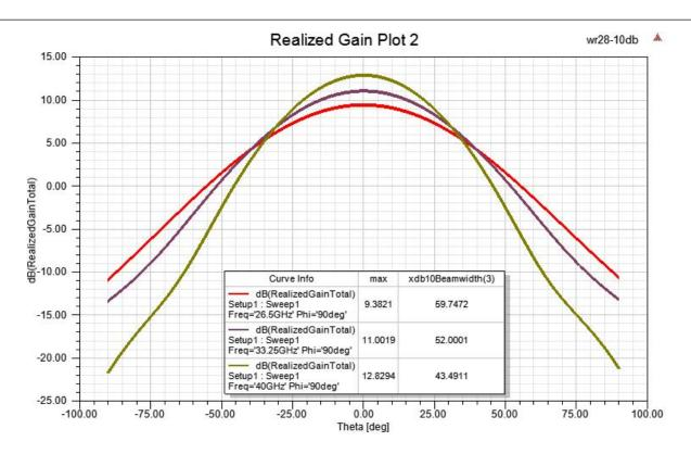
WR-28 Waveguide Antenna, 26.5 GHz to 40 GHz Frequency Range, 10 dBi Gain, UG-599/U Flange with Pre-Installed L mount from Fairview Microwave is in-stock and available to ship same-day. All of our RF/microwave products are available off-the-shelf from our ISO 9001:2008 certified facilities in Lewisville, Texas. Fairview Microwave is RF on-demand.
