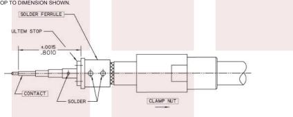
INSERT FORWARD INSULATOR INTO CONNECTOR IN ORIENTATION SHOWN. INSERT CABLE/ CONTACT SUB-ASSEMBLY INTO CONNECTOR UNTIL SEATED AND TIGHTEN CLAMP NUT TO 35-45 IN-LBS.
