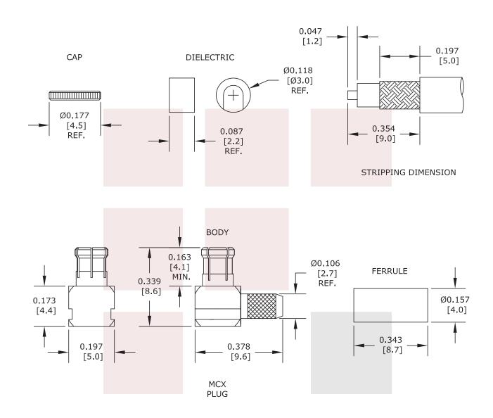
$\begin{array}{l} \underline{\text{STANDARD TOLERANCES}} \\ .X & \pm 0.2 \\ .XX & \pm 0.1 \\ .XXX & \pm 0.05 \end{array}$
