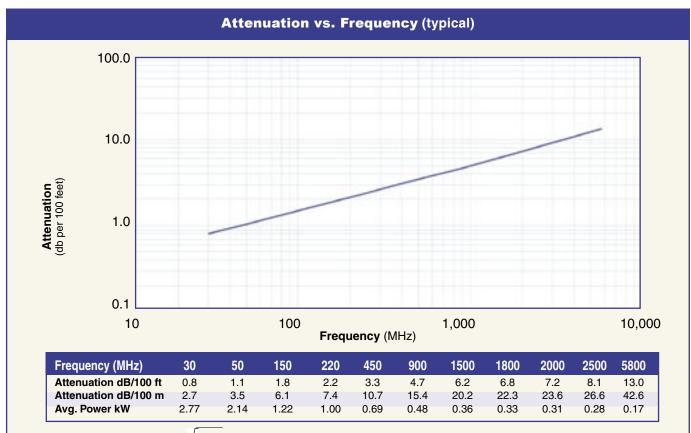
Calculate Attenuation = (0.146748) • √FMHz + (0.000312) • FMHz (interactive calculator available at http://www.timesmicrowave.com/cable\_calculators)
