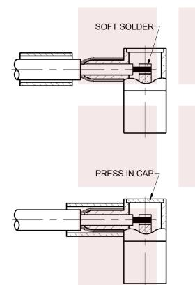
2.) INSTALL CABLE INTO BODY ASSEMBLY SO THE TUBE PORTION OF THE BODY SLIDES UNDER THE CABLE BRAID. PUSH CABLE FORWARD UNTIL CENTER CONDUCTOR IS IN SLOT OF CONTACT AND CABLE BRAID MEETS CONNECTOR BODY. SOFT SOLDER CENTER CONDUCTOR IN PLACE.
