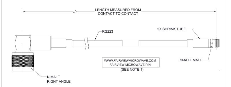
NOTES: CABLES 36" AND UNDER HAVE 1 LABEL CENTERED. CABLES OVER 36" HAVE 2 LABELS, ONE AT EACH END 6.0" FROM THE FRONT OF THE CONNECTOR.
