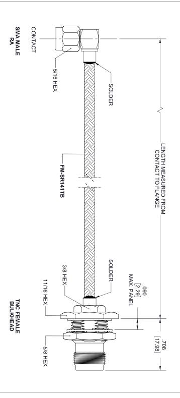
Ø .505<sup>+.005</sup><sub>-.000</sub>  $\begin{bmatrix} 12.83^{+0.13} \\ 0.00 \end{bmatrix}$ **MOUNTING HOLE**  $.472^{+.005}_{-.000}$   $\left[11.99^{+0.13}_{-0.00}\right]$
