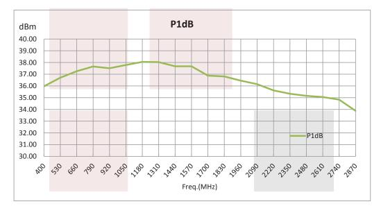
High Power Amplifier at 5 Watt P1dB Operating From 500 MHz to 2.8 GHz with 37 dB Gain, 52 dBm IP3 and SMA from Fairview Microwave is in-stock and available to ship same-day. All of our RF/microwave products are available off-the-shelf from our ISO 9001:2008 certified facilities in Allen, Texas. Fairview Microwave is RF on-demand.
