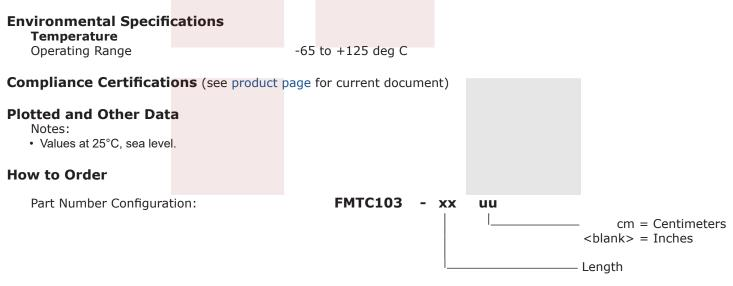
Example: FMTC103-12 = 12 inches long cable FMTC103-100cm = 100 cm long cable
