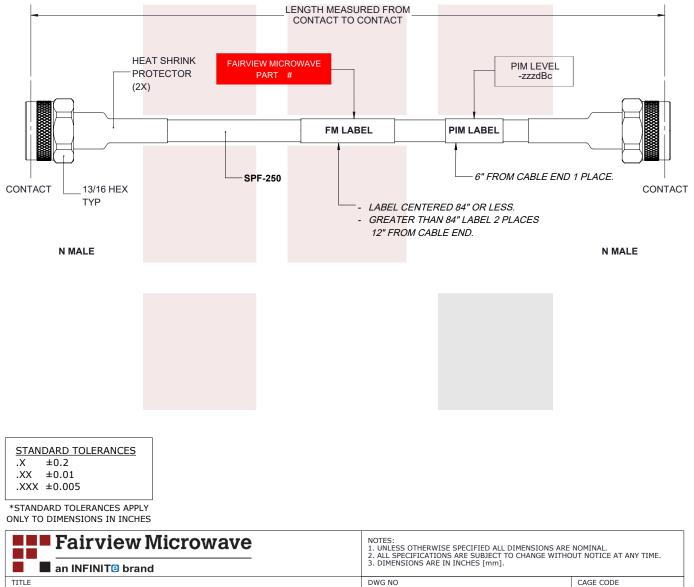
Fire Rated Low PIM N Male to N Male Cable SPF-250 Coax Using Times Microwave Parts
