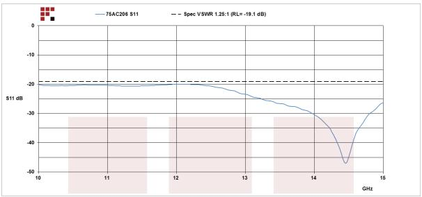
WR-75 to SMA Female Waveguide to Coax Adapter Square Cover Flange With 10 GHz to 15 GHz Frequency Range For X-Ku Band from Fairview Microwave is in-stock and available to ship same-day. All of our RF/microwave products are available off-the-shelf from our ISO 9001:2008 certified facilities in Allen, Texas. Fairview Microwave is RF on-demand.
