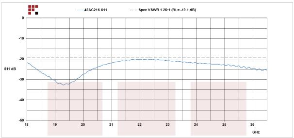
WR-42 to 2.92mm Female Waveguide to Coax Adapter Square Cover Flange With 18 GHz to 26.5 GHz Frequency Range For K Band from Fairview Microwave is in-stock and available to ship same-day. All of our RF/microwave products are available off-the-shelf from our ISO 9001:2008 certified facilities in Allen, Texas. Fairview Microwave is RF on-demand.
